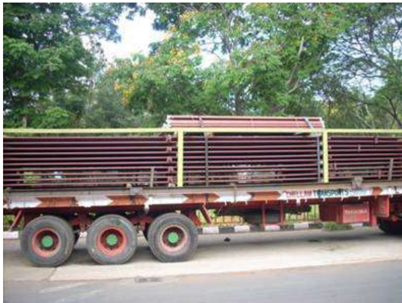
Example of improper loading of a tube bundle over a well-crated coil.
