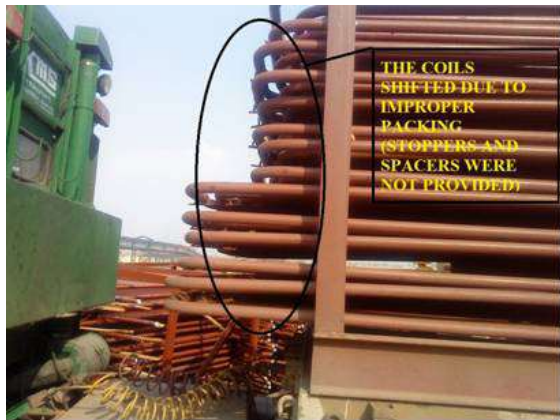
Example of the effect of not providing stoppers and spacers .... The coils slide in transportation and reach site like this.
