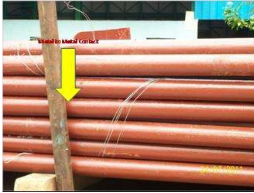
Improper metal to metal contact, which can cause rubbing of tubes
