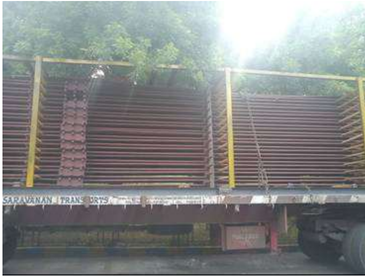
An example showing improper chain lashing - on the coil tubes, causing it to bend
