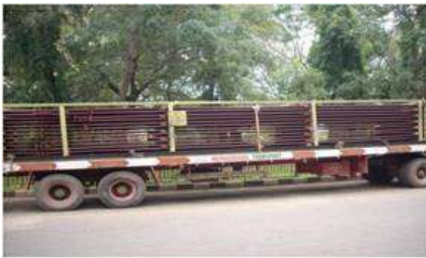
Example of nylon lashing. Nylon lashed drum ... but with an unacceptable chain lashing in the middle
