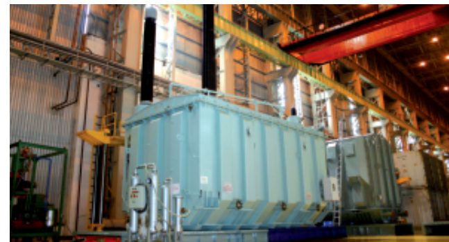
First indigenously built 1200 kV, 180 MVA Transformer in India, manufactured by BHEL
