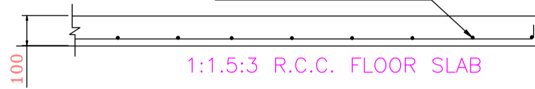
RCC FLOOR SECTION
