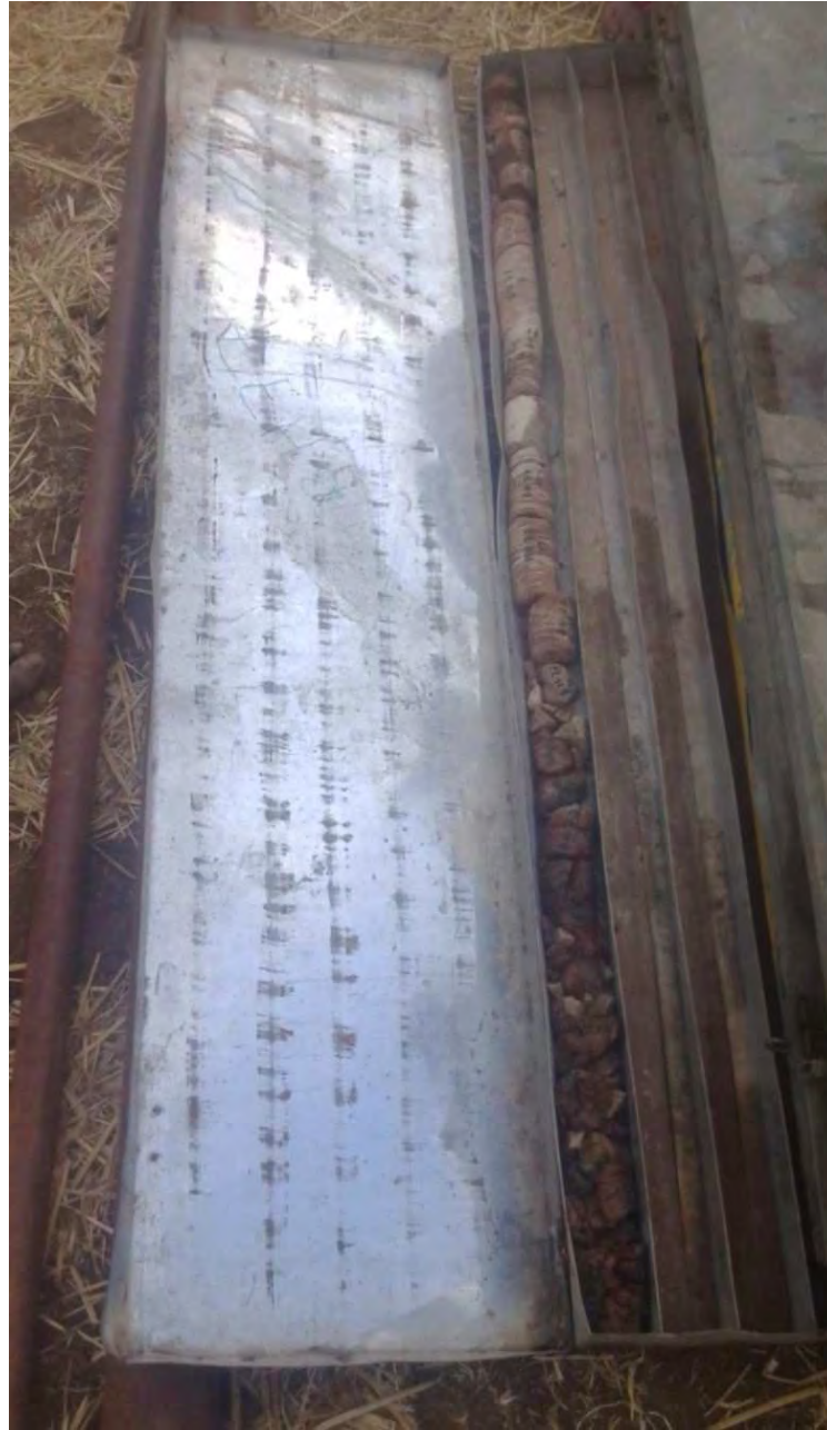
PHOTOGRAPH SHOWING CORE PIECES IN CORE BOX
